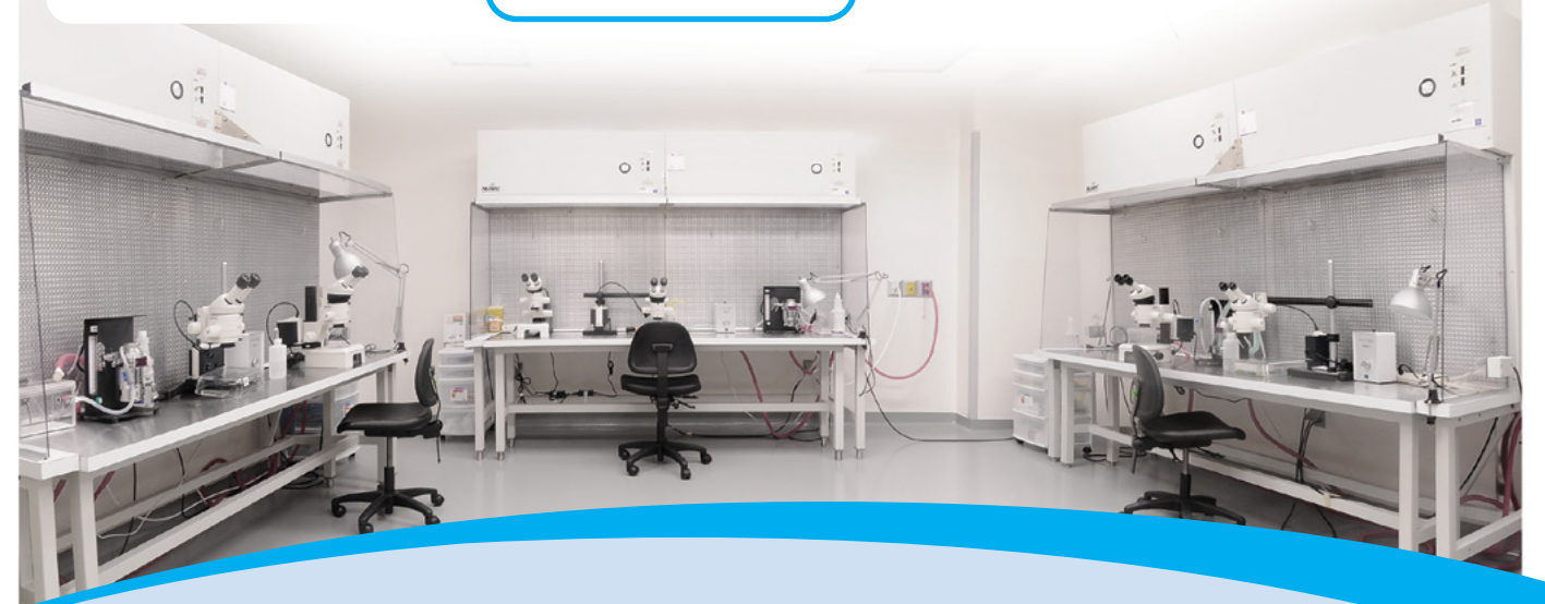
A custom model NU-240 was designed to offer a broader and taller work zone to accommodate a single workflow process involving microscopes. A customized isolation table was added to eliminate vibration in the work surface. The extended work surface allows a technician to perform several protocols without having to leave the work zone.
