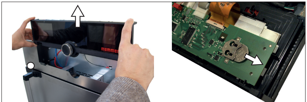
Fig. 25 Removing the lithium battery
